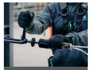
**No Sweat Tensioning** Locking and tensioning mechanisms are on the same side no need to travel back and forth during set up.
